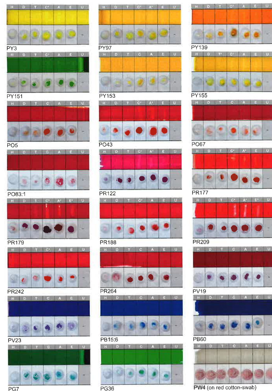
Fig. 4 The action of solvents in combination with mechanical stress to oil paint films with organic pigments can be regarded as dramatic. Due to the small particle size, even "insoluble" pigments will be extracted. Polar solvents seem to cause the most damage. (H = n-hexane; D = diethyl ether; T = toluene; C = chloroform; A = acetone; E = ethanol, U = untreated)
