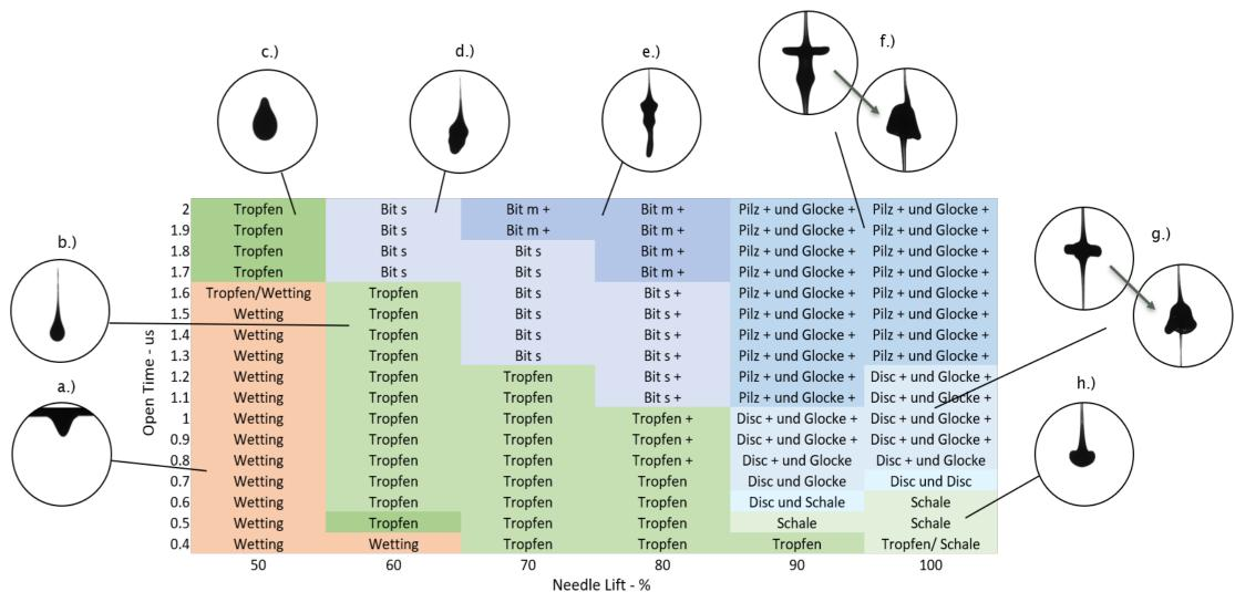
Jetting drop shape analysis for dispenser suitability characterization with focus on cocoa butter suspension-, emulsion and micro-foam systems
