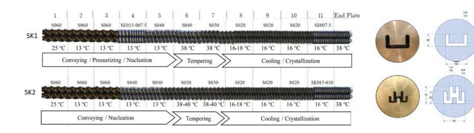
Twin screw extruder setup for the macro-printer with die geometries for the chocolate extrusion
