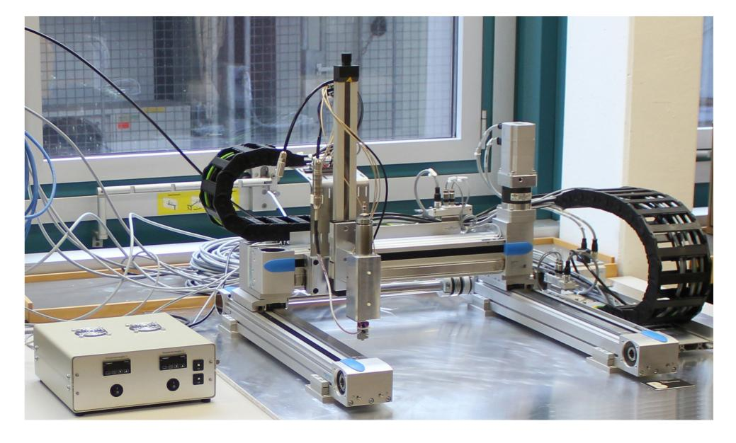
Additional flavoured chocolate in solid or foamed low-calorie form is applied by micro-extruder (meso) or printed as dots by micro-valve (micro) on the profile IDT 3D-dotting platform at ETH consisting of a robot, a controlling software, a micro valve and a temperature-controlled cartridge for high pressures (up to 20bar)
