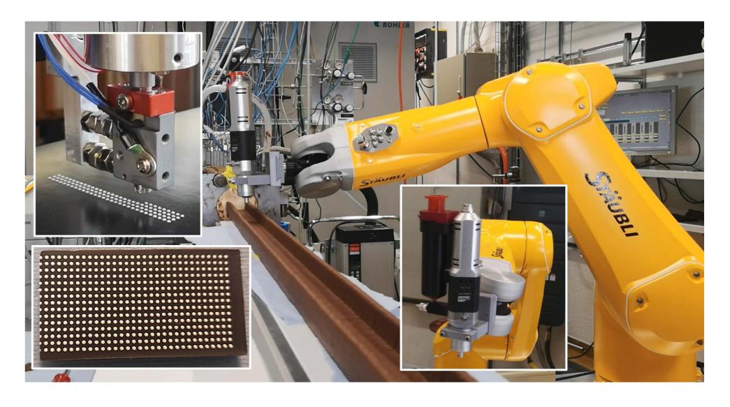
Ensemble of macro/meso/micro-scale print setups (a) Micro-nozzle, (b) Viscotec meso-print extruder, (c) Bühler macro-print extruder, (d) aroma/flavor dots
