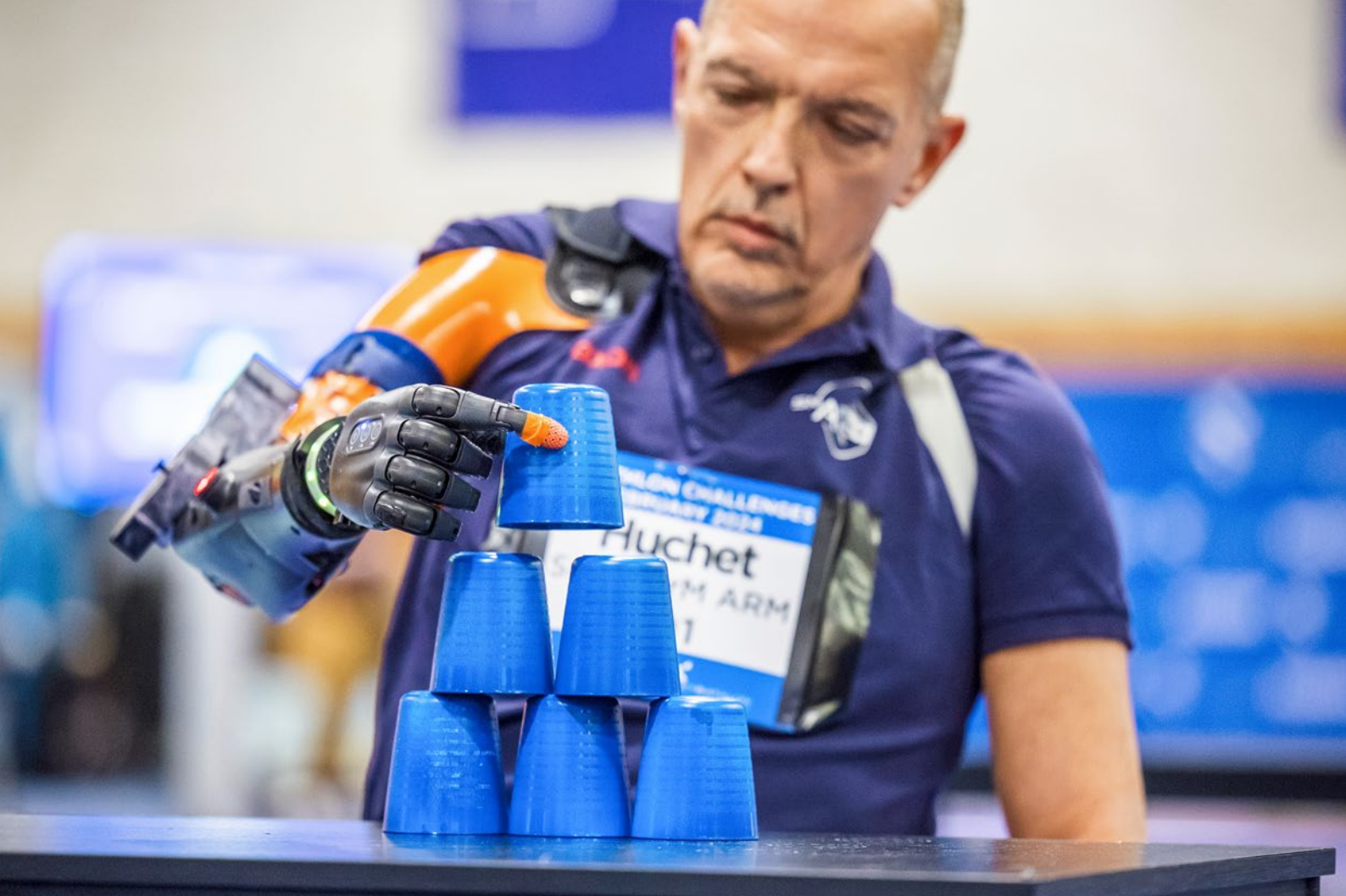
A major challenge: the prosthetic arm must be able to lift heavy objects and enable fine motor movements. (Fotos: ETH / Cybathlon / Alessandro Della Bella)
