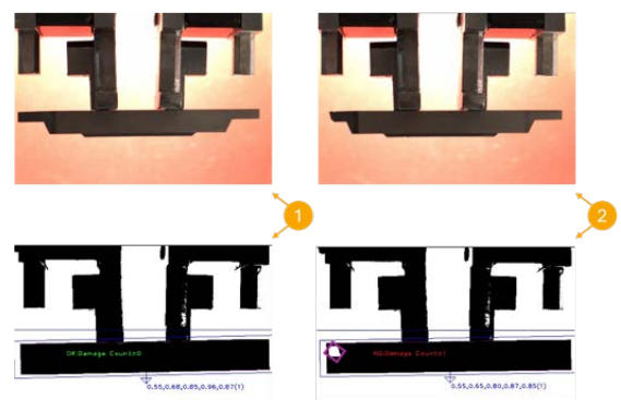
Figure 2: Images from the external camera. Top: Raw image. Bottom: Inspection results, (1) good part, (2) defective part.
