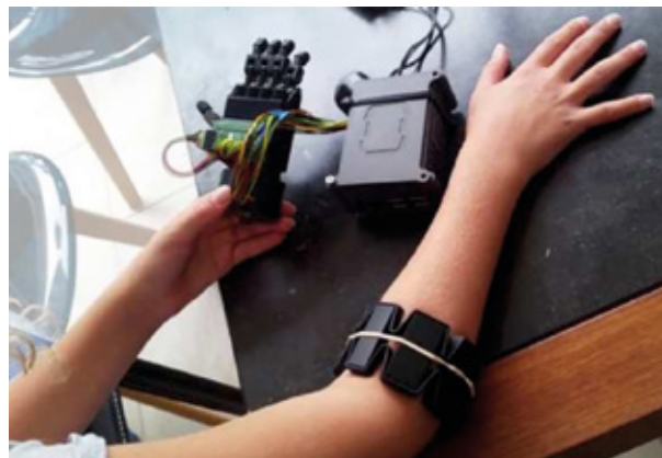
Realized prototype low-cost hand prosthesis. Size comparison between the hand of a 9-year-old child and the prosthesis. The prosthesis is controlled intuitively by reading EMG signals near the elbow.
