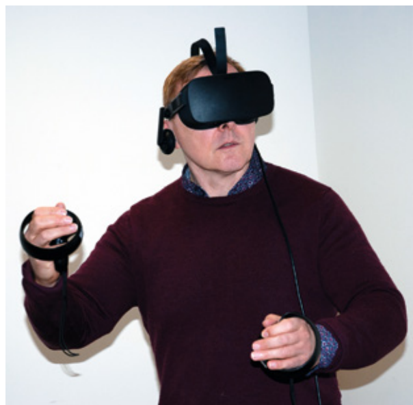
Virtual reality set-up for immersion in realistic scenes and interaction with avatars. The head-mounted display is equipped for eye tracking.
