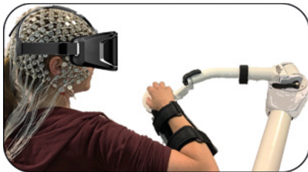
Robot-assisted arm training in virtual reality and recording of brain activity with EEG electrodes placed on the head
