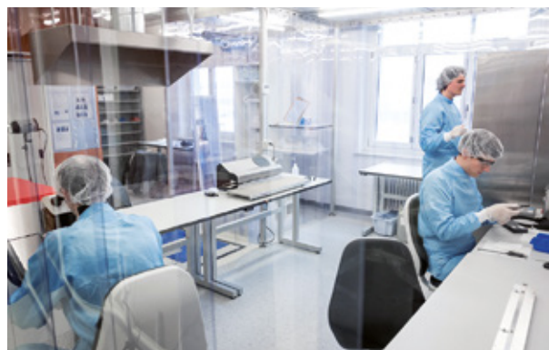
HuCE at the BFH Centre for Technologies in Sports and Medicine has setup and runs a certified clean room qualified as ISO class 7, used for medical device manufacturing at Switzerland Innovation Park, Biel/Bienne.
