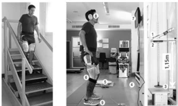
Left: Walking downstairs; Right: (1) electromagnet, (2) falling barbell weight, (3) stopper, (4) wire rope, (5) force transducer, (6) brace, (7) monitor for feedback, (8) headphones and attenuator, (9) force platform.
