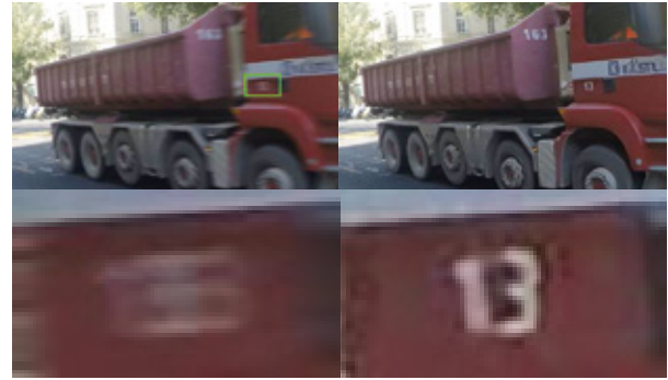
Example of a motion blurred image of a moving object (left). Learned from a large database of blurred and sharp image pairs, we are able to invert the blurring process and restore the sharp texture details such as the text shown here.
