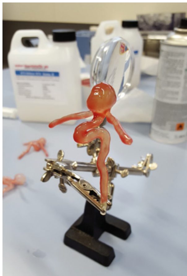
Ultra-thin silicon layered, single-patient customized aneurysm model.
