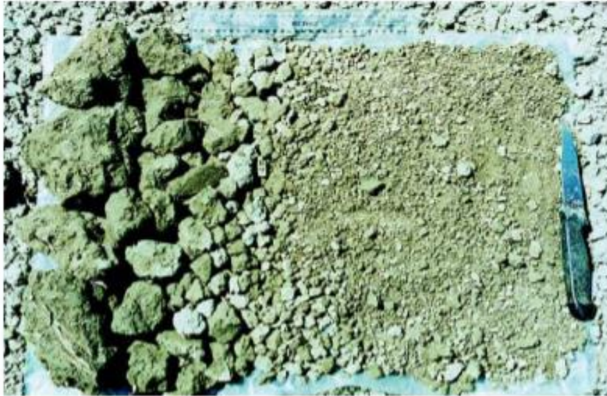
MODERATE CONDITION VS = 1 Soil contains significant proportions of both coarse firm clods and friable, fine aggregates
