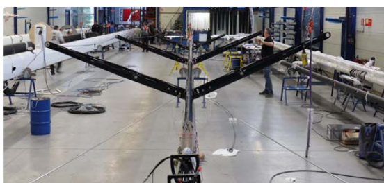
All of the parts are made of carbon fibre-reinforced plastic, and the manufacturing process is manual.
