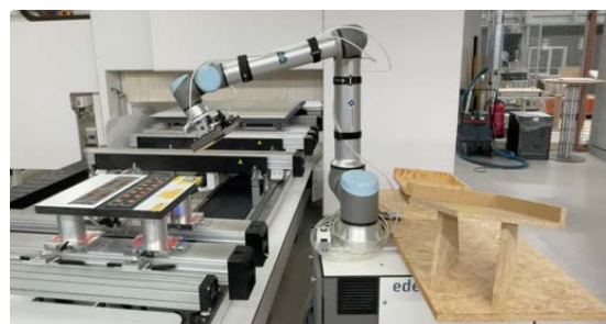
Cobot-AMR system loading a CNC-Machine
