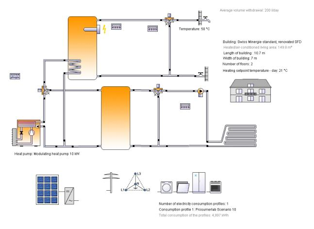
Fig. 3: Configuration of Polysun used for in the Prosumer-Lab test bench for the main scenarios.
