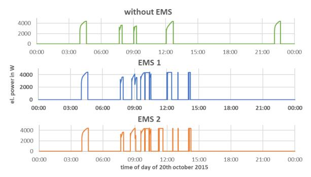
Fig. 5: Comparison of power consumption of the heat pump during operation without control and when controlled by two different EMS.
