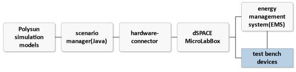
Fig. 2: Integration of Polysun to the Prosumer-Lab HIL test bench. The device under test is an energy management system which communicates with other test bench devices and the scenario manager.
