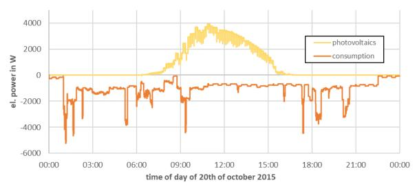
Fig. 4: Power flows of a representative 4-person household in Switzerland on 20 October 2015, divided into production by photovoltaics and accumulated consumption.
